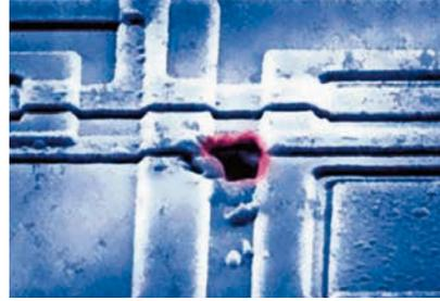
Figure 64 | Example of ESD damage
