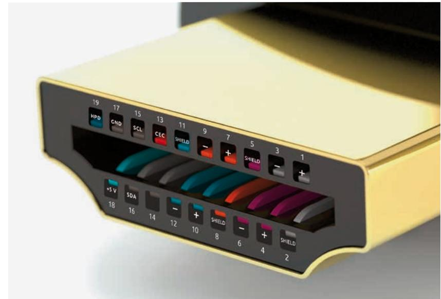
**Figure 81 | Pinout and front view of HDMI connector**
